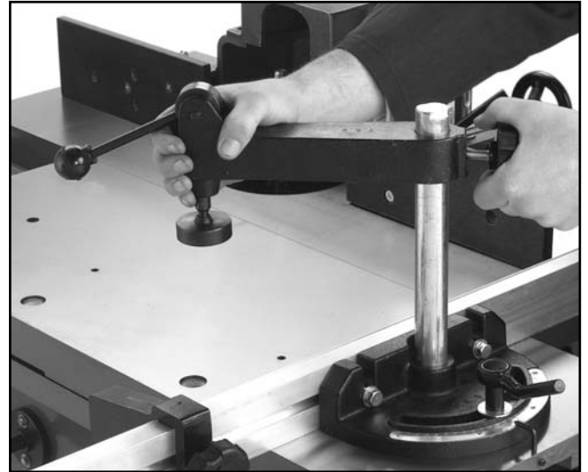
Figure 24. Installing the clamping unit.
